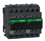
Reversing Contactor, TeSys Deca, 3P(3NO), AC-3, <=440V, 32A, 230V AC 50/60Hz coil, with electrical interlocking, screw clamp terminals
